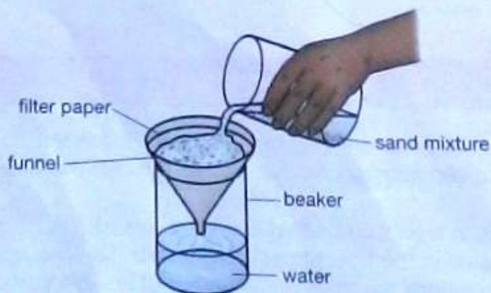
Figure 8.4 Separating a mixture of sand and water by filtration
