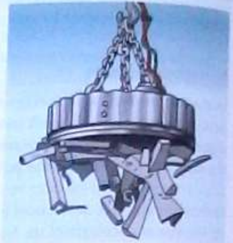
Figure 18.4 Cranes use electromagnets to lift and drop scrap metal.
