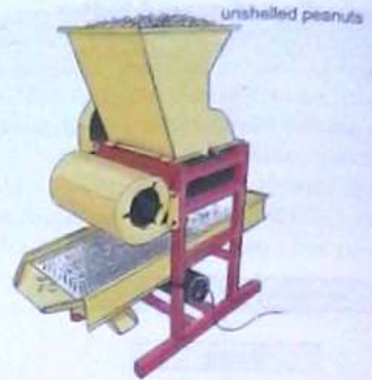
Figure 11.3 A peanut shelling machine
