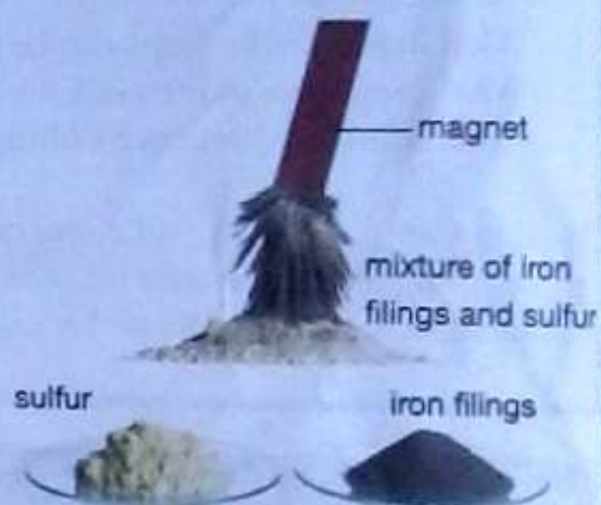
Figure 8.5 Separating iron and sulfur with a magnet
