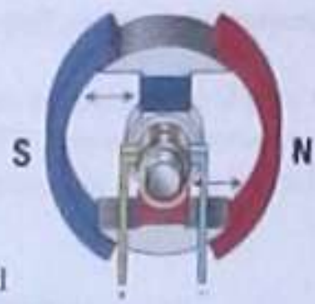
Figure 18.3 C-magnets are used in motors.
