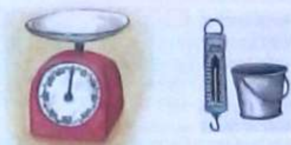
Figure 15.5 The two types of spring balance
