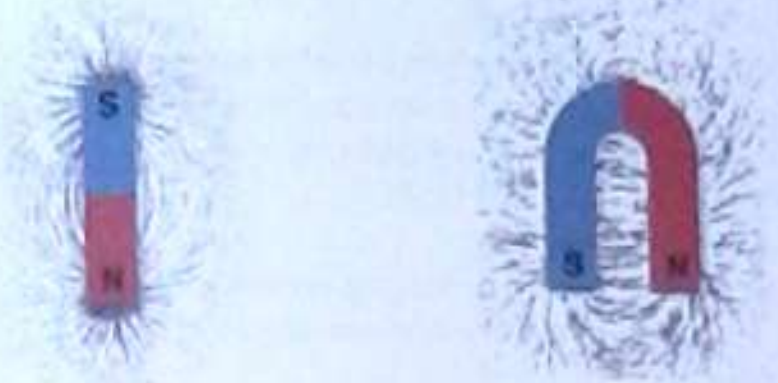
Figure 18.8 The magnetic field lines of a) a bar magnet and b) a horseshoe magnet
