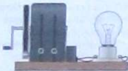
Figure 17.11 Using a dynamo to light a bulb
