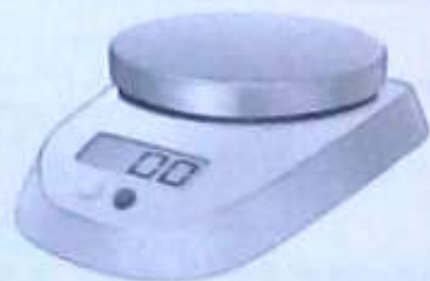
Figure 15.20 Digital balance that has been zeroed
