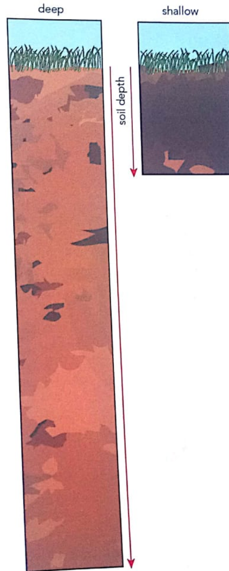
Figure 3.10 A very deep, and a very thin or shallow soil profile compared
