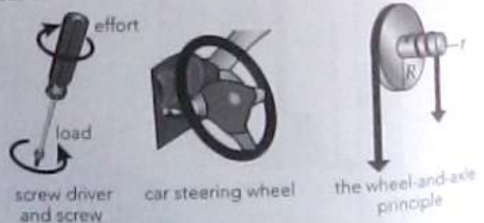
Figure 19.9 Some wheel-and-axle systems
