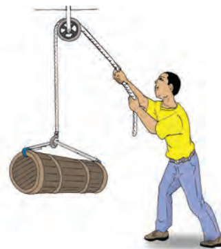
A man using a pulley to lift a heavy object
