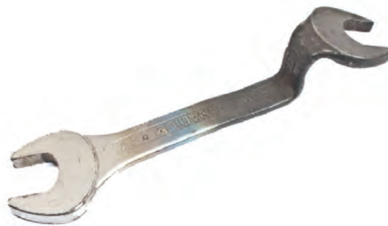
Spanner modified by bending
