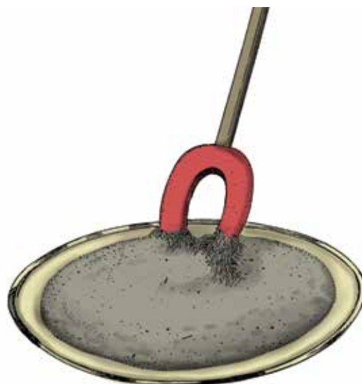
Figure 5.1 A mixture of sand and iron filings can be separated by using a magnet.
