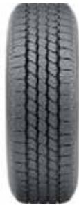
Figure 3.11 The tread of the tyre increases the friction between the tyre and the road surface
