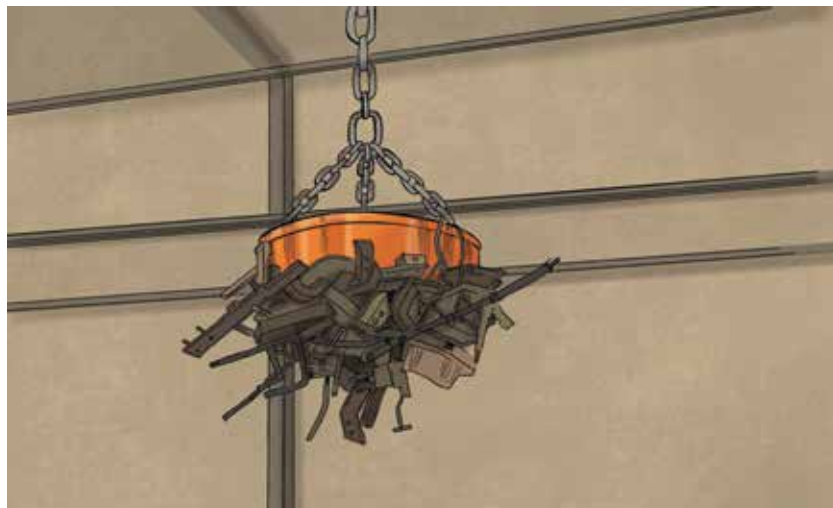
Figure 1.4 Magnetism can be used to remove steel cans from other general recycling
