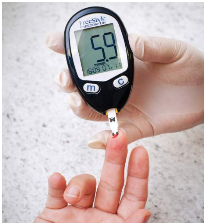
Figure 14.28 Biosensors use biological materials, such as enzymes, to measure the concentration of molecules such as glucose. This glucose biosensor is used to check the glucose concentration in a sample of blood. The meter shows a reading in the normal range.
