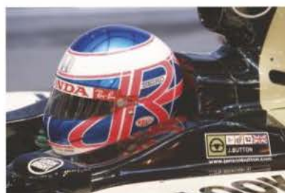
▲ Figure 7 Formula 1 drivers' helmets need to be lightweight as the less weight it adds to a drivers head, the smaller the risk of whiplash injuries under the extreme G-forces experienced in accelerating and braking. Helmets worn by racing drivers contain Kevlar which is five times stronger than steel, weight for weight
