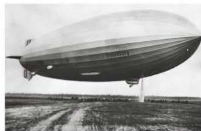
▲ Figure 1 The German airship Hindenburg held about 210\,000\text{ m}^3 of hydrogen gas
