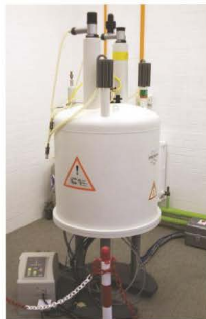
▲ Figure 4 Modern NMR instruments use electromagnets with superconducting coils to produce the strong magnetic fields required. The large white tank holds a jacket of liquid nitrogen surrounding an inner jacket of liquid helium which cools the magnet coils to 4 K
