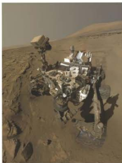
▲ Figure 6 The Mars Rover Curiosity carries a mass spectrometer to look for compounds of carbon that may suggest that there was once life on Mars.
