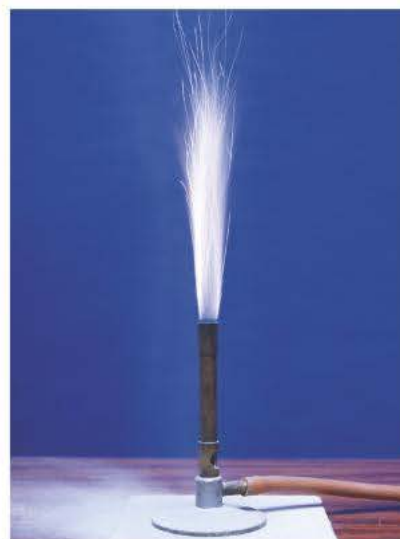
▲ Figure 2 Aluminium burning in oxygen from the air. Powdered aluminium is being sprinkled into the flame
