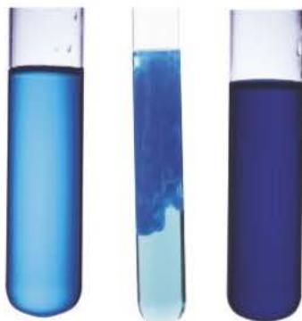
▲ Figure 1 Pale blue solution of [\text{Cu}(\text{H}_2\text{O})_6]^{2+} , the pale blue precipitate of [\text{Cu}(\text{OH})_2(\text{H}_2\text{O})_4] , and the deep blue solution of [\text{Cu}(\text{NH}_3)_4(\text{H}_2\text{O})_2]^{2+}
