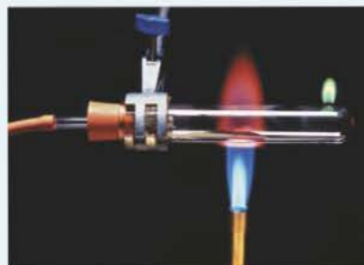
▲ Figure 1 Finding the empirical formula of copper oxide
