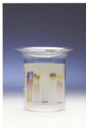
▲ Figure 1 The cellulose of the paper holds many trapped water molecules (the stationary phase). Here, ethanol is the mobile phase, or eluent
