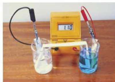
▲ Figure 4 Measuring the potential difference of zinc and copper
