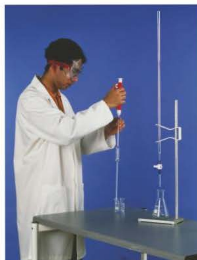
▲ Figure 1 An acid–base titration, to find the concentration of a base. A volumetric pipette is used to deliver an accurately measured volume of base of unknown concentration into the flask. The acid of known concentration is in the burette
