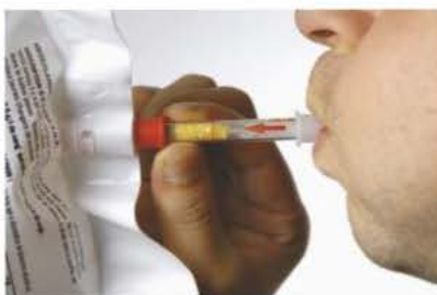
▲ Figure 6 A modern fuel cell breathalyser
