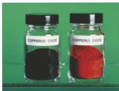
▲ Figure 1 The two oxides of copper – copper(II) oxide (left) and copper(I) oxide (right)
