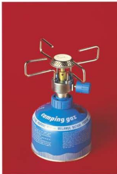
▲ Figure 1 Camping Gaz is a mixture of propane and butane. Polar expeditions use special gas mixtures with a higher proportion of propane, because butane is liquid below 272 K [−1 °C]
