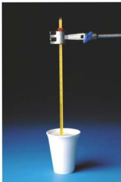
▲ Figure 6 Polystyrene beakers make good calorimeters because they are good insulators and have low heat capacities
