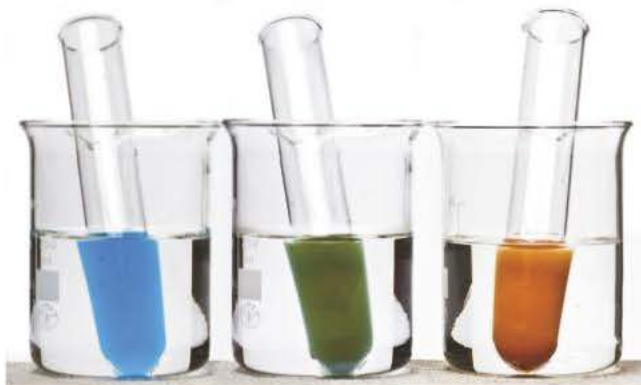
▲ Figure 2 When an aldehyde is warmed with Fehling's solution, the blue colour will turn green then a brick-red precipitate forms
