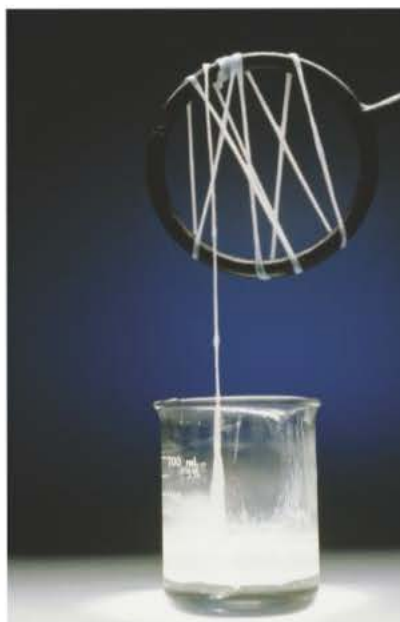
▲ Figure 6 When 1,6-diaminohexane and hexane-1,6-dioyldichloride meet, Nylon-6,6 is formed at the interface. This demonstration was first performed by Stephanie Kwolek who developed Kevlar
