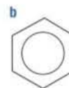
▲ Figure 3 Aromatic compounds are based on the benzene ring C_6H_6 . Although it appears to have three double bonds as in a , the electrons are spread around the ring, making it more stable than expected. It is usually represented as in b
