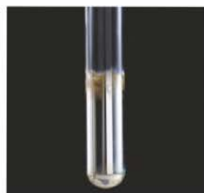
▲ Figure 3 The reaction of aldehydes with Ag^+ ions was once used as a method of silvering mirrors.
