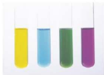
▲ Figure 2 Zinc ions in acid solution will reduce vanadium(V) through oxidation states V(IV) and V(III) to V(II). The final flask is normally stoppered because oxygen in the air will rapidly oxidise V(II)
