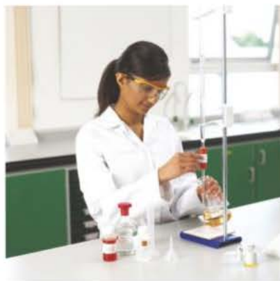
▲ Figure 1 Titrating the ethanoic acid to investigate the equilibrium position
