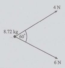
A particle of mass 8.72 kg is pulled horizontally at a constant speed of 5 ms<sup>-1</sup> along a rough straight road by two horizontal forces of 4 N and 6 N inclined to each other at 60°, (see diagram).
