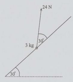
A ring of mass 3 kg is threaded on a rough wire inclined at 30° to the horizontal. The ring is about to slip down the wire when a force of 24N inclined at 30° above the wire is applied to it, (see diagram).
