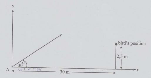
A stone is projected from point A with a speed of 20 ms<sup>-1</sup>, at an angle of 30° to the horizontal, towards a bird 30 m away. The bird is standing on a a pole 2,5 m vertically above the level ground (see diagram).
