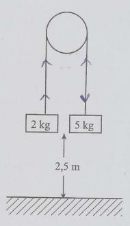
Masses of 2 kg and 5 kg are connected by a light inextensible string and hang vertically on either side of a smooth pulley. The system is released from rest with both portions of string vertical and both particles at a height of 2,5 metres above the ground (see diagram).
