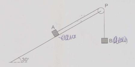
A light inextensible string is attached to A and passes over a small smooth pulley P fixed at the top of the inclined plane. To the end of the string is attached a particle B of mass m which hangs freely.
