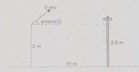
The initial speed of the ball is V ms<sup>-1</sup> at an angle of elevation  $\arcsin\left(\frac{\sqrt{3}}{2}\right)$ , and the ball moves freely under gravity.
