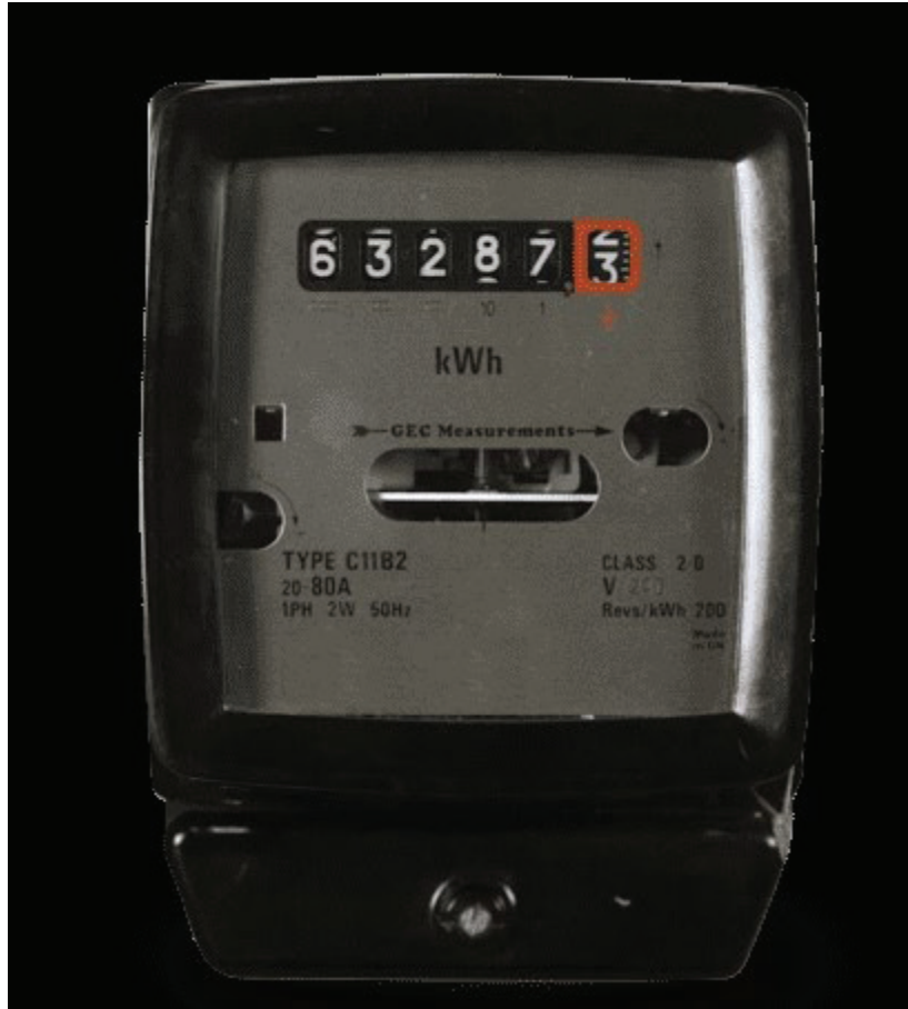
Fig. 29.3 Electricity Meter (Source npower.com)
