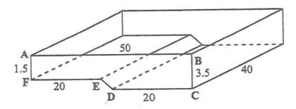
The diagram shows a swimming pool of uniform cross-section ABCDEF, of length 50 m and breadth 40 m.
