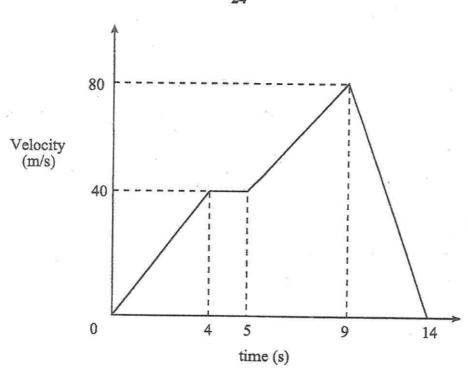
The diagram is the velocity – time graph for an electric train. The train accelerates uniformly from rest until it reaches a speed of 40 m/s in 4 seconds. It maintains this speed for a second before accelerating again for a further 4 seconds. After reaching a speed of 80 m/s, it decelerates to rest in 5 seconds.
