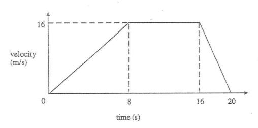
The diagram shows the velocity-time graph of a body which accelerates uniformly from rest to 16 m/s in 8 seconds, travels at constant velocity for a further 8 seconds and finally retards uniformly to rest in 4 seconds.
