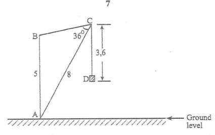
In the diagram, ABC is a crane lifting a load D. AB and BC are beams and ACD is a string. Given that the vertical beam AB = 5 m, AC = 8 m. CD = 3.6 m and BCA calculate
